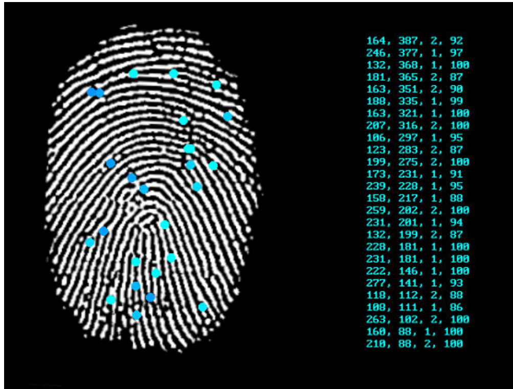
Fig 2. Characteristic points together with their coordinates, type code (ridge ending or bifurcation) and color-coded likelihood. The machine also prints this information on a card, a probabilistic IDcard for your reference.
